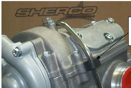
Install the rubber anti-vibration block on the oil supply tube as shown
