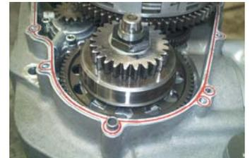
Use care to avoid damage to the end of the crankshaft.
