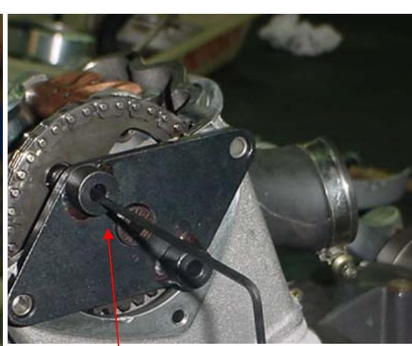
Insert a screwdriver to know the holes are aligned
